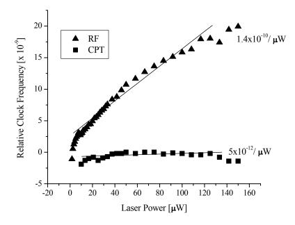
Figure 11: Light shift of RF and CPT interrogation
