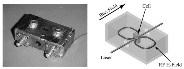
Figure 7: 9.2 GHz RF resonance cavity
