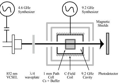
Figure 4: Schematic of dual-mode CSAC testbed
