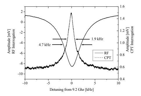
Figure 8: Typical RF spectra
