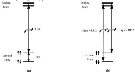
Figure 1. Relevant energy levels for (a) RF and (b) CPT interrogation
